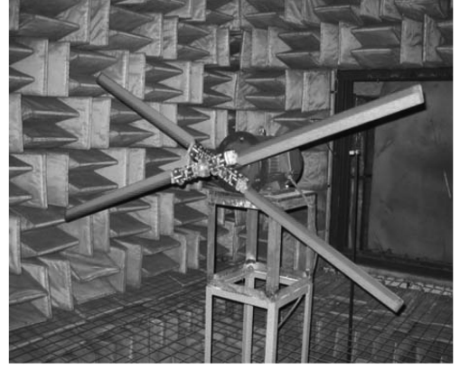
Fig. 6 Noise experiments on scissors rotor in anechoic aeroacoustic laboratory.
